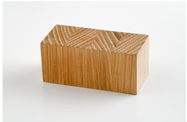
Figure 10. Two RFID tags laminated between four sections of oak.
