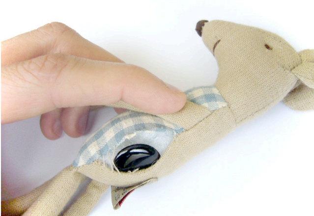
Figure 8. Stitching RFID tag inside toy mouse.
