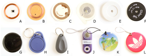
Figure 2. Passive RFID technology from raw, unprotected circuitry through various protective encapsulations towards simple packaging.
