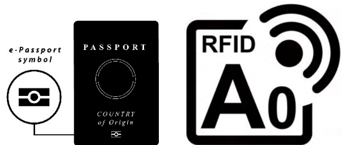
figure 4. Icon for RFID-based passports (left). figure 5. Icon for AIM Global EPC RFID tags (right).
